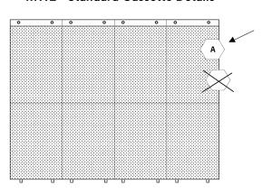
Place the BAUX Acoustic Wood Wool according to the picture. They should not be placed further out than Detail A
